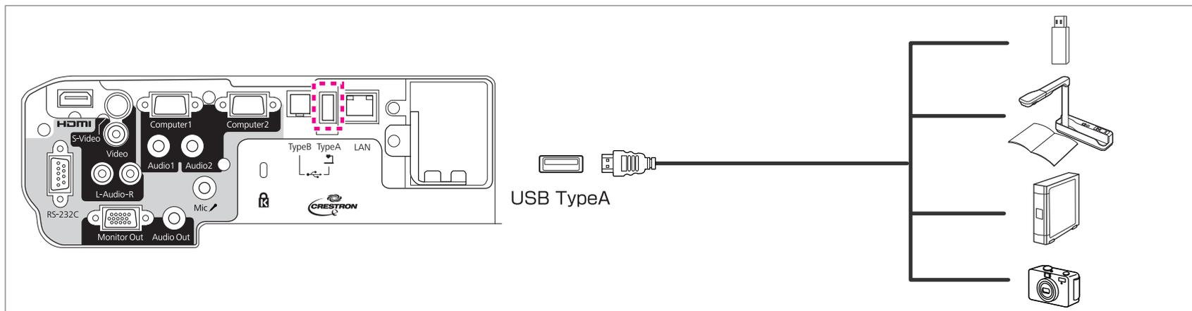
When the USB device is connected, you can project image files on the USB memory or digital camera using Slideshow.
