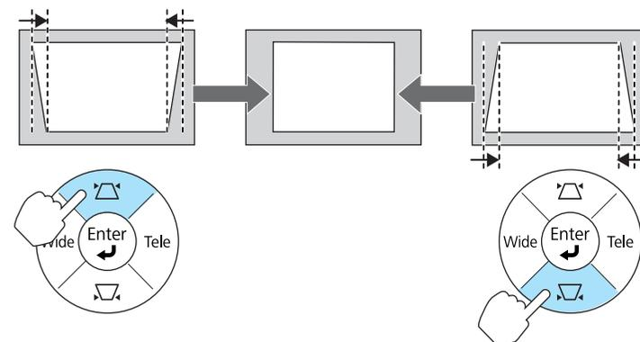
Press the [Tele] or [Wide] buttons to correct horizontal distortion.
